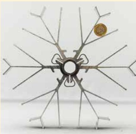
Fig. 3 Through the axially finned tube, steam flows through the latent heat storage tank at high pressure. The heat is transferred to the salt via the fin structure.
