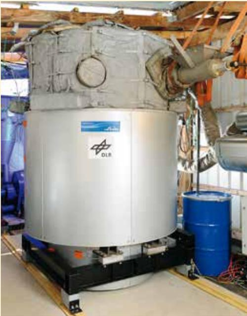
Fig. 2 The figure shows the investigated latent heat storage tank on a pilot scale.
