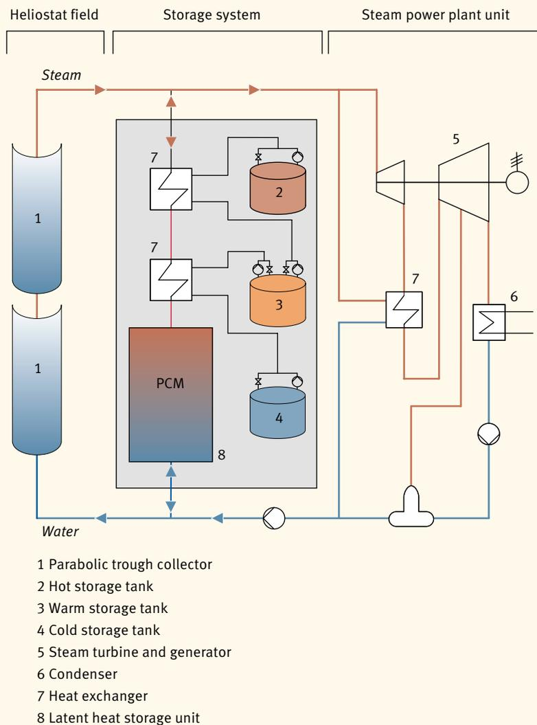
Fig. 1 Integration of the storage cascade system into a parabolic trough power plant with direct steam generation.
