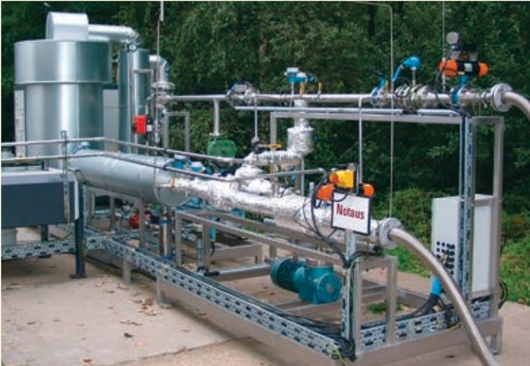
**Fig. 3** The research team tested both catalytic separation on activated aluminium oxide (cat-ox process) and adsorptive purification using activated carbon with subsequent regeneration (activated carbon process).
