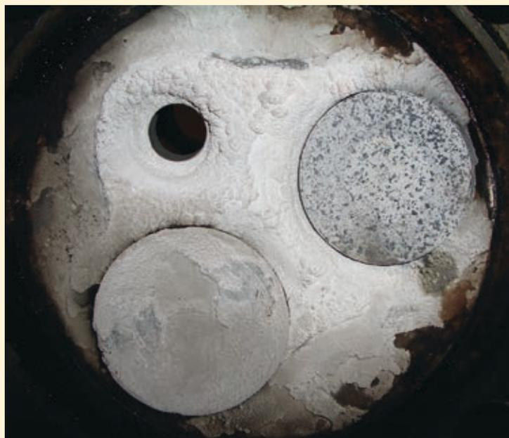
Fig. 2 Silicon dioxide deposits on the cylinder head of a gas motor after 3,500+ operating hours resulting from the combustion of organic silicon trace compounds in the engine compartment.
