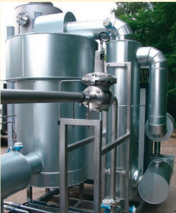
**Fig. 4** The two materials, aluminium oxide and activated carbon, were each examined by the research team in an isolated fixed-bed reactor with landfill gas.
