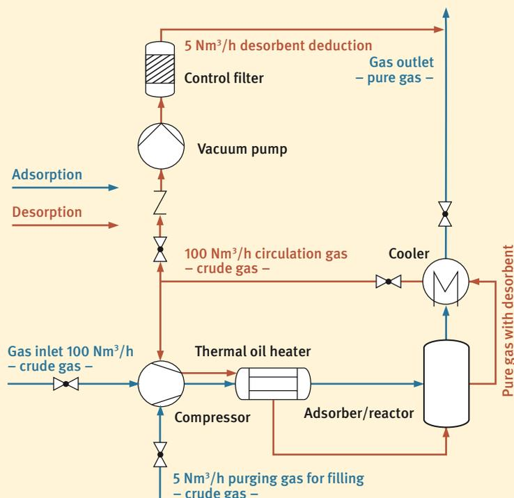
Fig. 1 Diagram illustrates the test structure of the 100-Nm<sup>3</sup>/h plant at the Vereinigte Ville landfill site.
