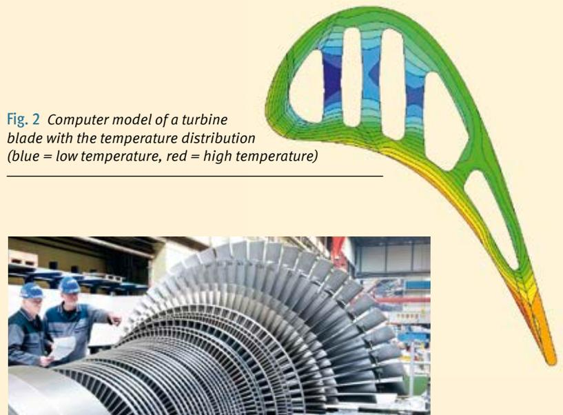
Fig. 2 Computer model of a turbine blade with the temperature distribution (blue = low temperature, red = high temperature)
