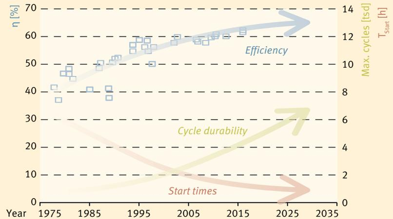
Fig. 1 Since 1975, the efficiency ( $\eta$ ), start times and the maximum cycle durability have improved considerably in power plants with gas and steam turbines (CCPP).
