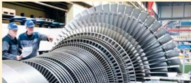
Fig. 3 A single-chamber industrial steam turbine for power generation with an output of 80 MW
